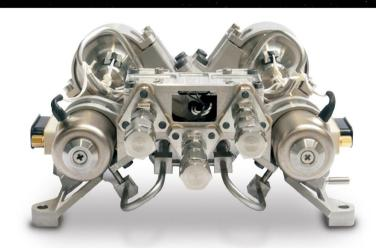
Bradford's Flow Control Unit (FCU) technology provides precise control of the xenon propellant flow rates to ion thrusters. The FCU makes use of proportional flow control valves to precisely control the flow rate of xenon by controlling the pressure differential over a fixed hydraulic resistance (i.e. thermally controlled flow restrictor). In principle one of two control logics can be applied:
