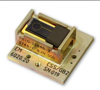
The Cosine Sun Sensor (CoSS) delivers coarse information about the position of the sun relative to the spacecraft. This information is used for coarse maneuvering of the spacecraft and to inform the spacecraft about the position of the sun.
