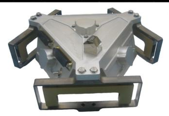
The Acceleration Measurement Unit (AMU) is an independent measurement unit. The AMU is composed of four accelerometers disposed on a regular tetrahedron. It includes an accelerometer adaptation electronic board with four electrically independent channels connected to each Fibre Optic Gyro (FOG) Electronic Module (FEM) of the Gyro Electronic Unit (GEU) by an electrical harness.
