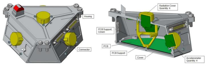
The figure above shows the AMU mechanical structure without the titanium isolators. It is composed with four independent channels with four accelerometers disposed on a regular tetrahedron.
